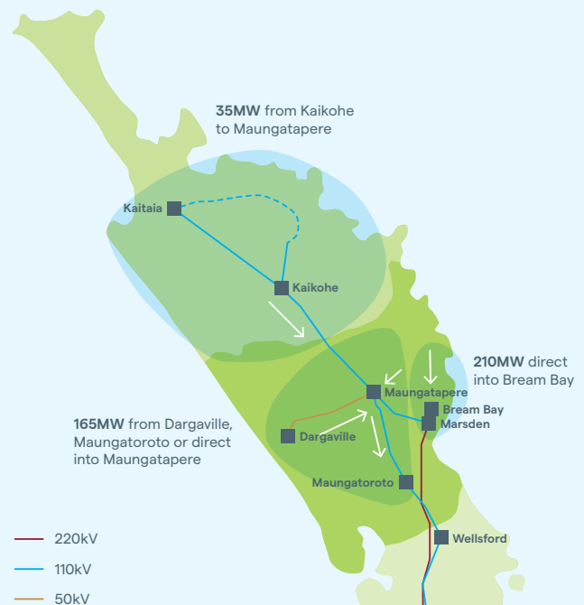
Figure 8: Illustration of existing network export capacity
